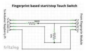
Fig. 12. Fingerprint Based Start/Stop Touch Switch
