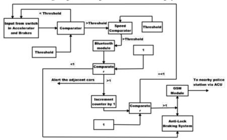
Fig. 4.Signal flow diagram of Rash Driving Alerting System
