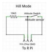
Fig. 10. Circuit diagram for interfacing Altitude sensor for Hill Mode
