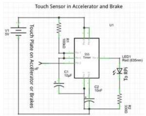
Fig. 10. Circuit Diagram of Touch Sensor or Switch in Accelerator or Brakes
