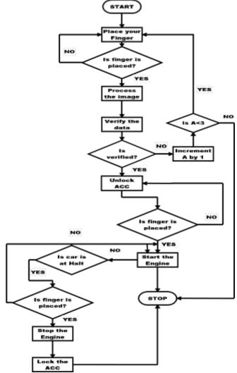
Fig. 7.Flow chart of Fingerprint based start/stop Touch Switch
