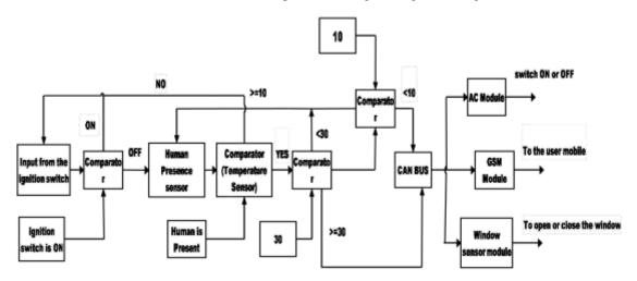
Fig. 3. Signal Flow Diagram of Child in Car Alerting System
